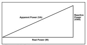
**Figure 1.2**: Relationship between apparent, real and reactive power
